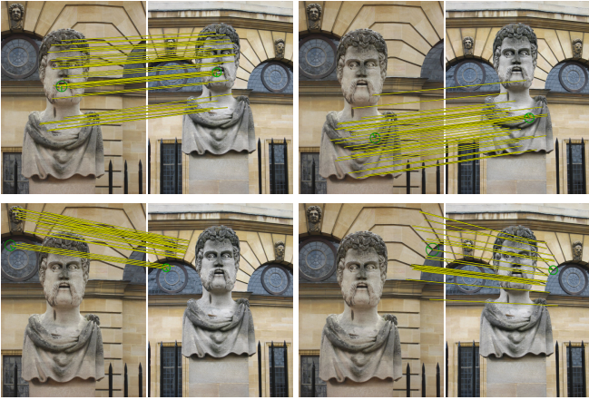
Figure 4: Left: Tentative correspondences with SURF features and a 100K vocabulary. Right: Inliers using FastSM. As revealed in Figure 5, there are two different matching surfaces between the two images, and two different relative transformations. FastSM captures only one.
