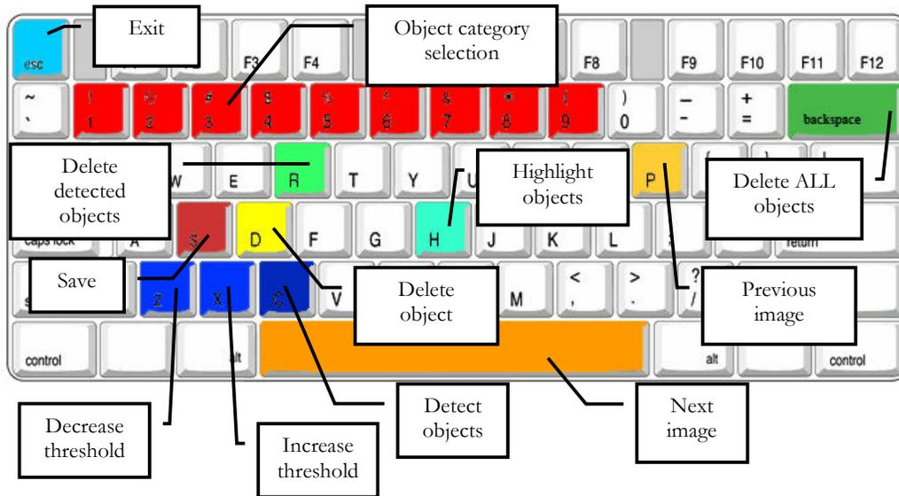
Fig. 4 : Keyboard functions.
