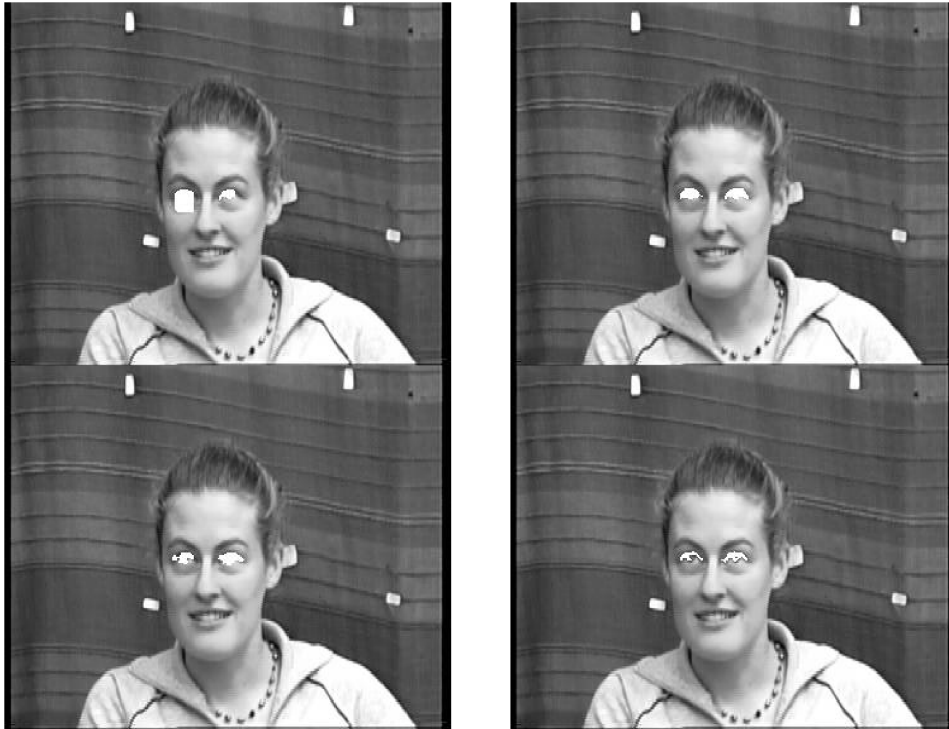
Figure 6 (a) Final mask for the eyes in frame A and (b) detected feature points on frame A
