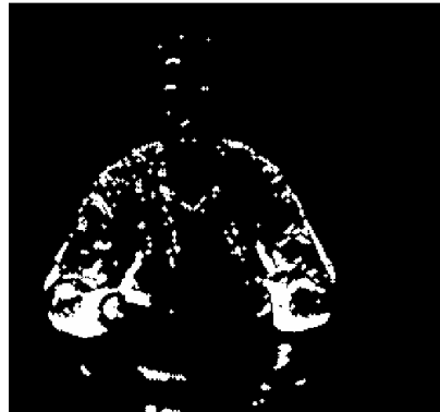
Fig. 10. Initial motion mask after pixel difference thresholded to 10% of maximum
